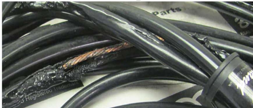
Fig. 2. Melted insulation on welding cable.
